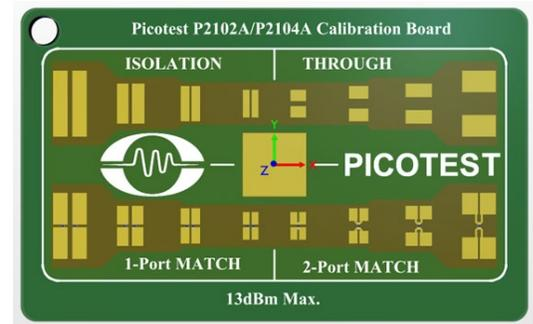
The P2104A includes a S-O-L-T and Isolation calibration board.
