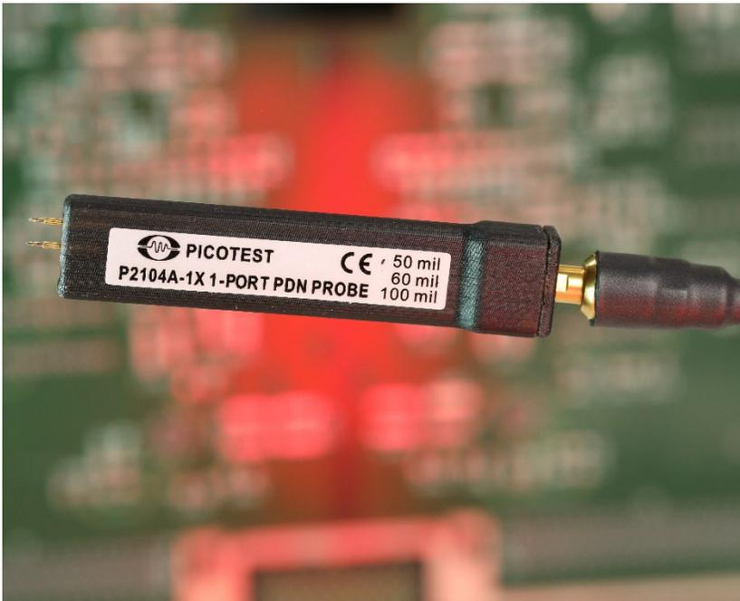
You can quickly characterize multiple VRMs to ensure stability, review rail impedance, check ripple, and even verify if your simulation model.
